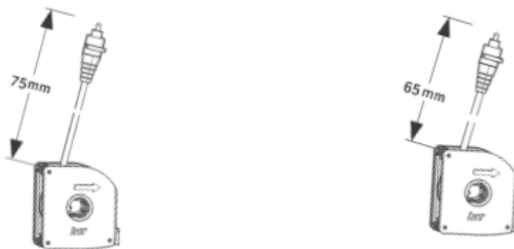
BOX132W-SS75 Standard tether assembly 2 core \phi 3.0mm 75 cm cable, outside cable 70cm
